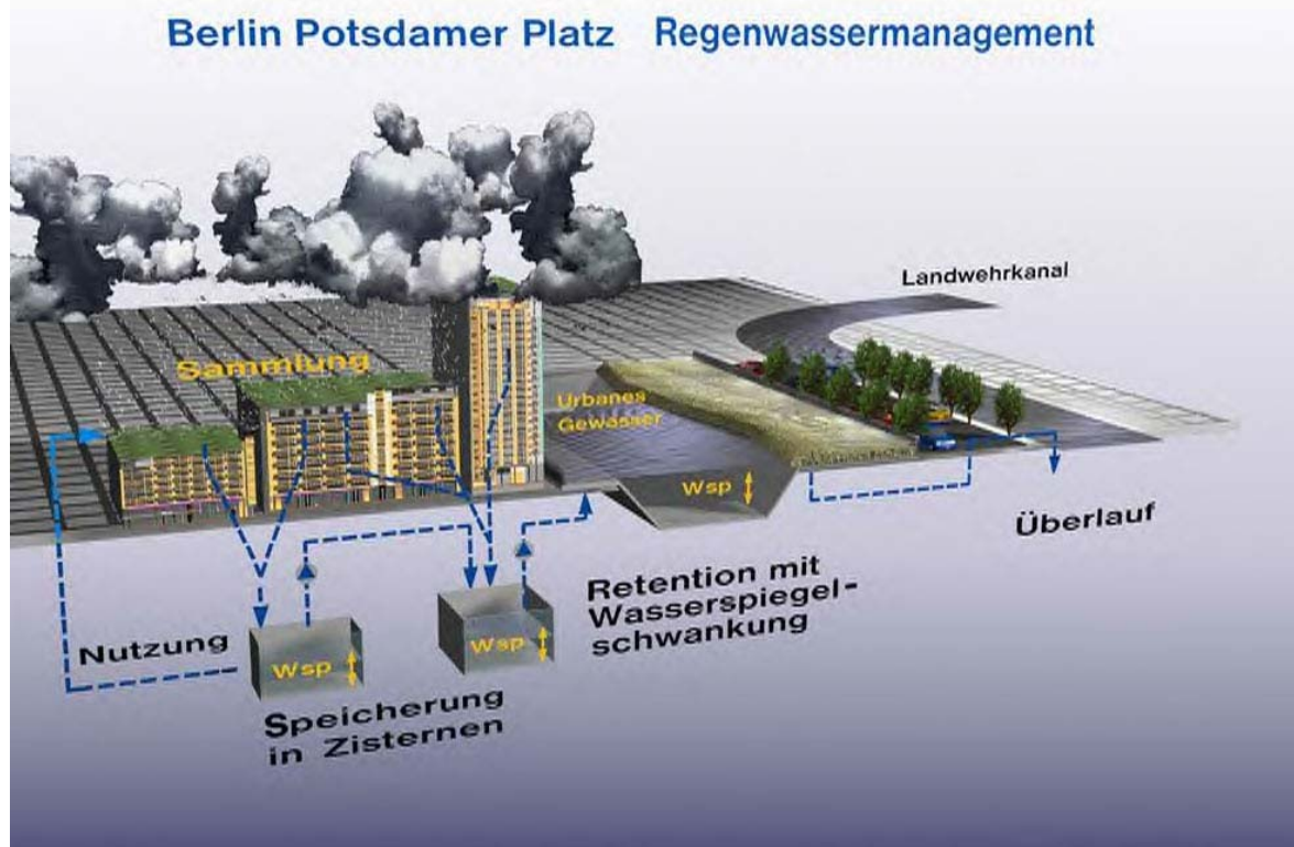
Figure 8.2 Potsdamer Platz Multi-layered Rainwater Management and Reuse System
