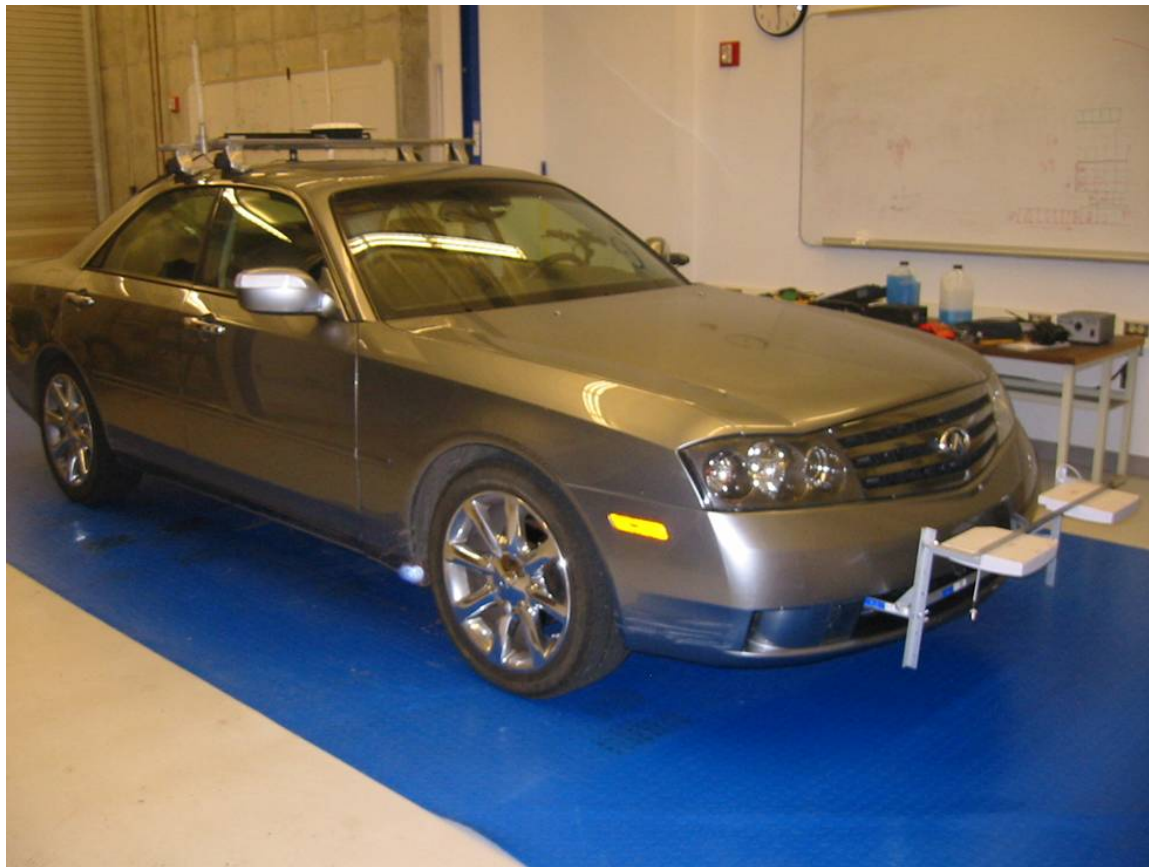
Figure 3.3: Test vehicle RFID reader antenna installation.
