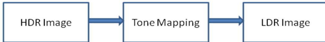
Figure 3.24: The whole scene is rendered using high dynamic range and then tone mapped to convert it to low dynamic range in order to be displayed on the monitor.
