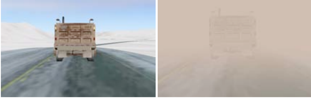
Figure 3.31: Experiments to test the effectiveness of lighting configurations on the back of snowplows are piloted with basic low-luminance contrast versus high-luminance contrast conditions. Normal snowplow lighting is used in both conditions.
