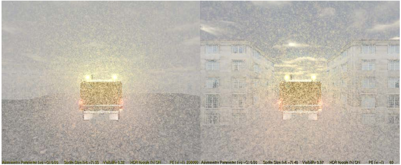
Figure 4.8: Snow model with Gaussian transparency, HDR rendering, aggregate snow and scattering effects.
