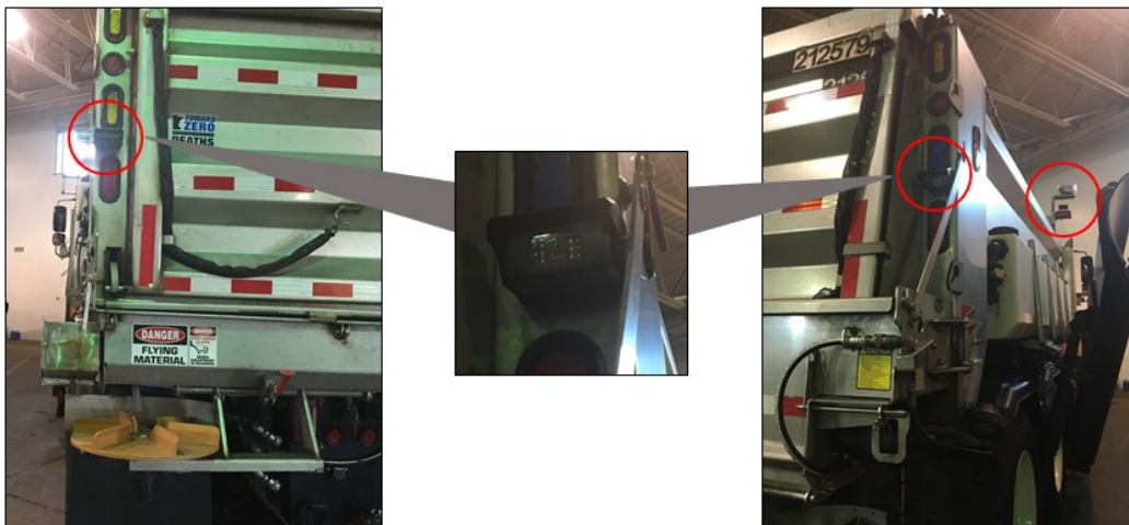
Figure 2.14. Rear left, rear right, and strobe mounted cameras.
