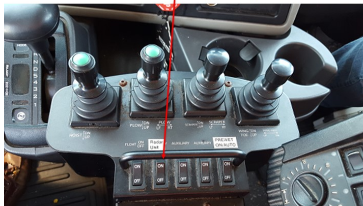
Figure 4.7 Location of the Power Switch to Turn on the Backup Assist System.
