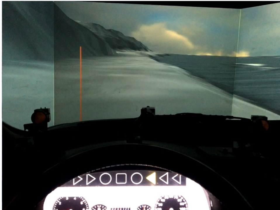
Figure 2.25. Operator perspective during the simulator plowing exercise using the LED guidance system with the road covered by snow.
