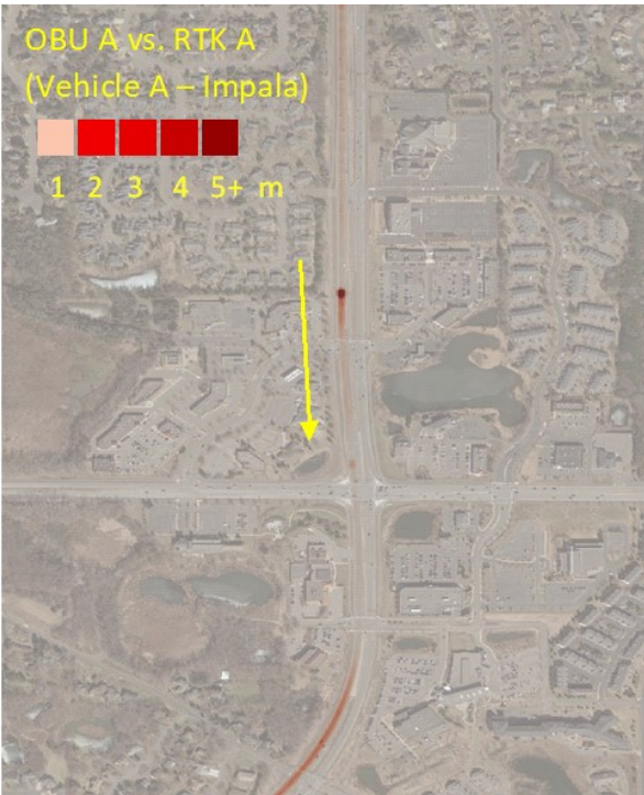
Figure 3.14. Position error of OBU vs. RTK based on vehicle trajectory (traveling SB on Radio Dr near Valley Creek Rd).
