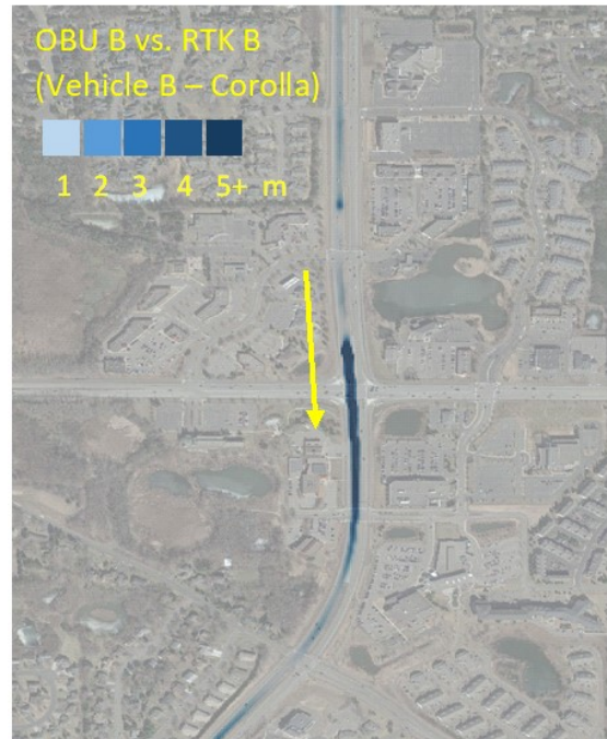
Figure 3.14. Position error of OBU vs. RTK based on vehicle trajectory (traveling SB on Radio Dr near Valley Creek Rd).
