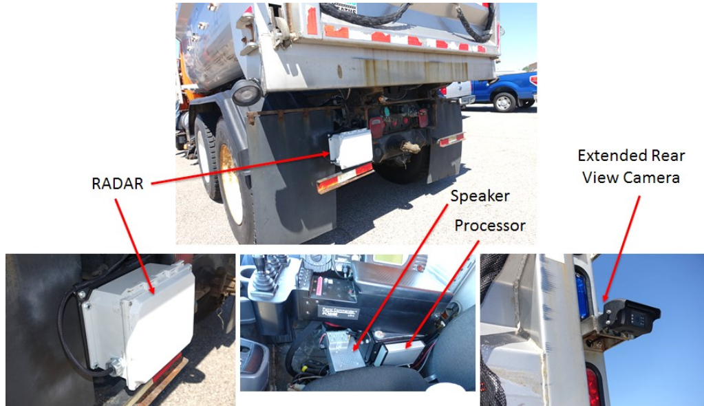
Figure 4.6 Backup Assist System Installed on Plow Truck #212570.
