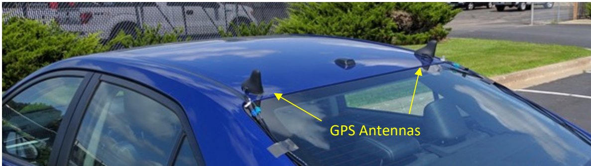
Figure 3.6. Savari GPS antennas installed in left-right configuration on the rooftop of a passenger vehicle.
