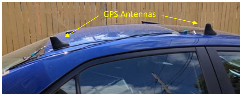
Figure 3.5. Savari GPS antennas installed in front-back configuration on the rooftop of a passenger vehicle.
