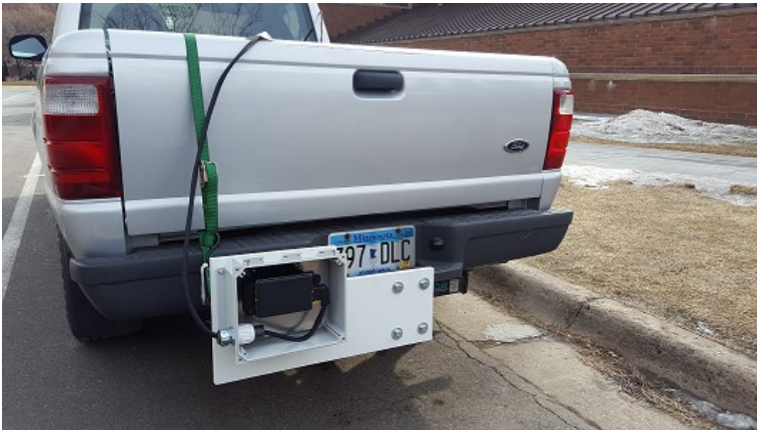
Figure 4.1 A radar based backup assistance system on a pickup truck.
