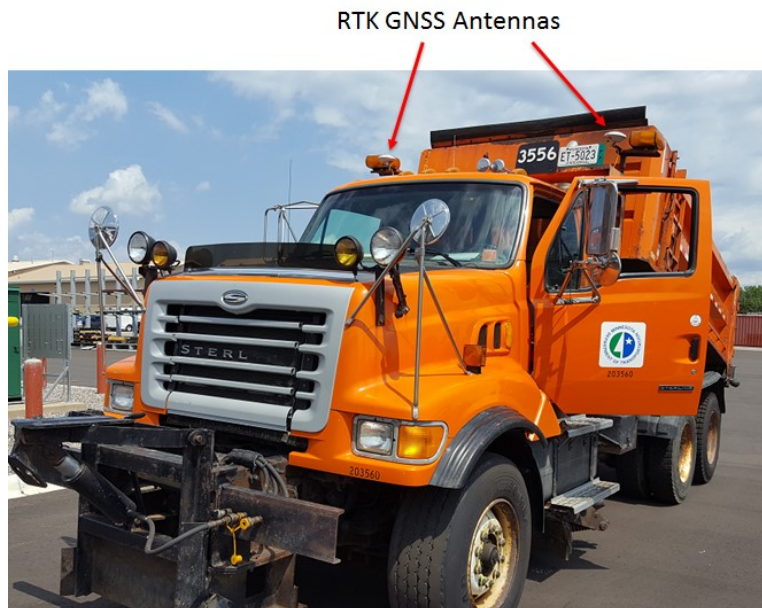
Figure 5.7 GNSS antennas installed on plow truck #203560.
