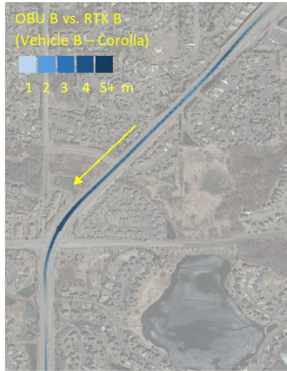
Figure 3.13. Position error of OBU vs. RTK based on vehicle trajectory (traveling SB on Radio Dr near Lake Rd).
