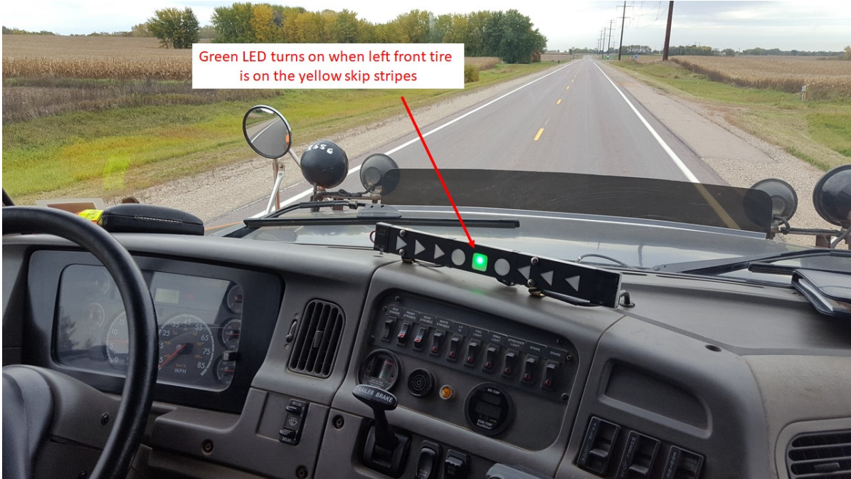
Figure 5.11 LED indication of the lateral position of the plow truck (10/13/2017).
