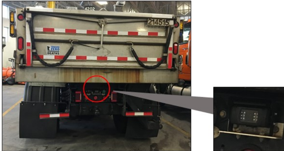
Figure 2.15. Rear-under bed mounted cameras.
