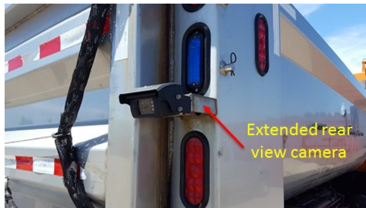
Figure 4.4 Extended rear view camera for better field of view.
