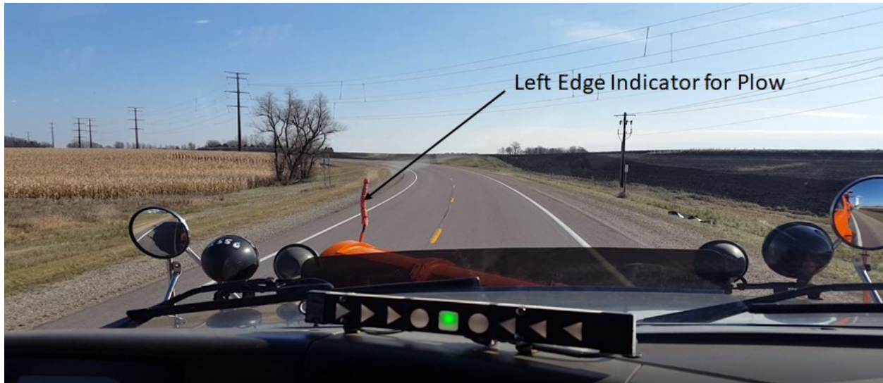
Figure 5.13 Test plow truck on MN-25 (11/7/2017).
