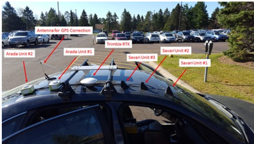
Figure 3.3. Installation of Arada & Savari GPS antennas on the rooftop of a passenger vehicle
