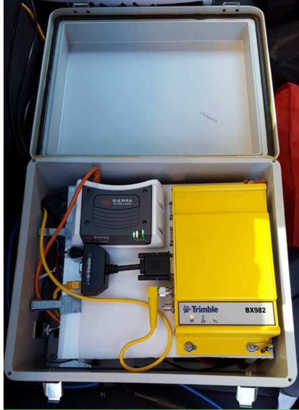
Figure 3.12. A portable RTK GNSS and DSRC OBU system.
