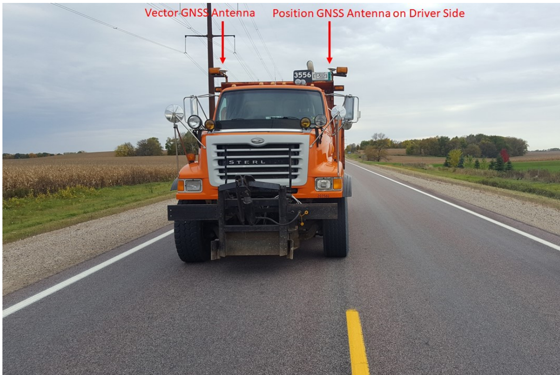
Figure 5.10 GNSS antenna mounting configuration on plow truck #203560 (10/13/2017).
