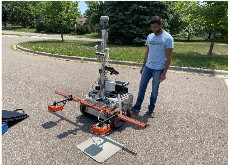
Figure A.9 Assembled robot; Operator performing GPR calibration.
