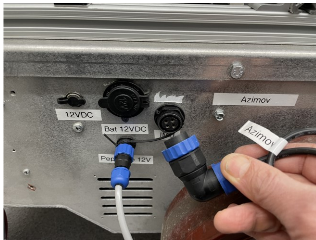
Figure A.5 Connecting an IMU cable to the robot.
