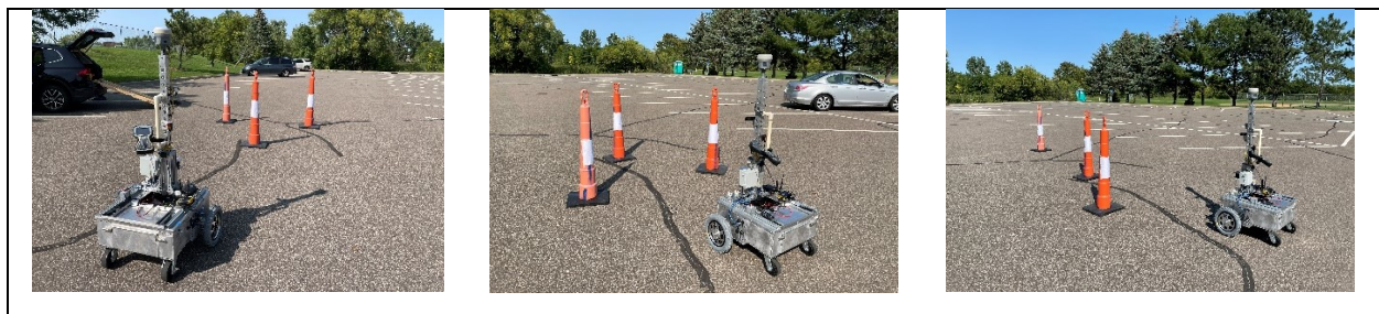
Figure 6.3: LiDAR and stereo camera static outdoor experiments using MnDOT traffic delineators.
