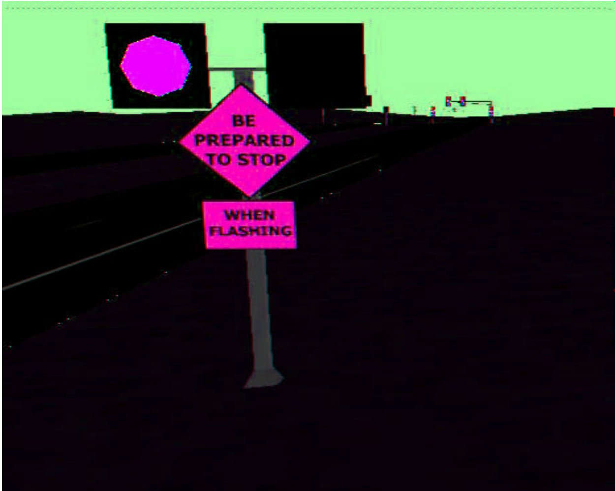
Figure 2-3. Perspective from SDTE showing simulated AWF in foreground, and simulated pole and mast arm with dual traffic signal in background.
