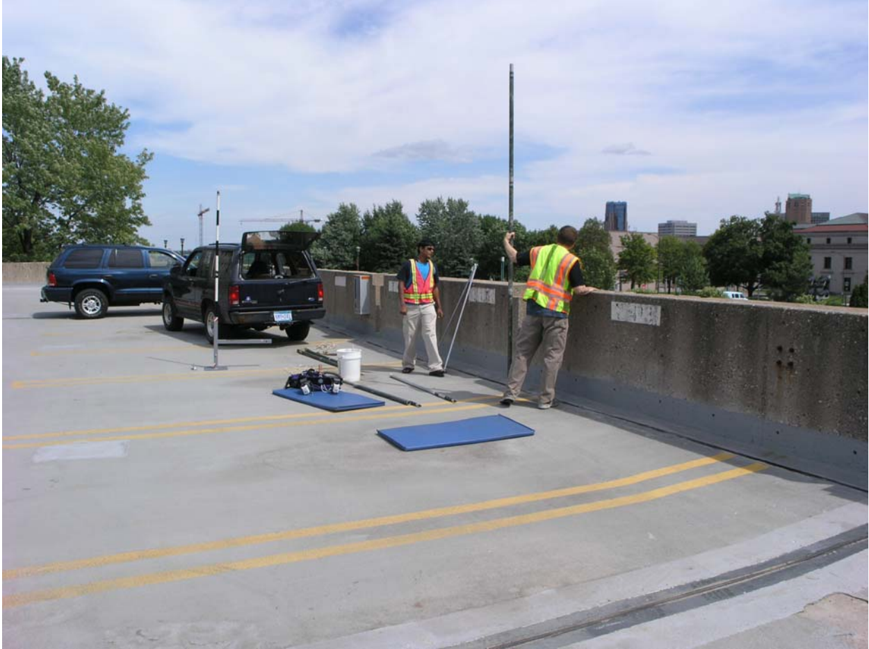
Figure E-2. Nesting boom tube elements and judging boom height that will be required for camera viewing of the crosswalk (at this site, the crosswalk is located below the second level of the parking ramp where the observation vehicle is positioned).
