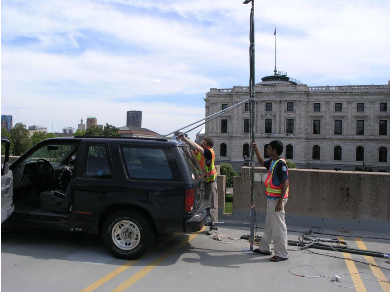
Figure E-5. Affixing diagonal support rods to camera boom and to luggage rack of observation vehicle.
