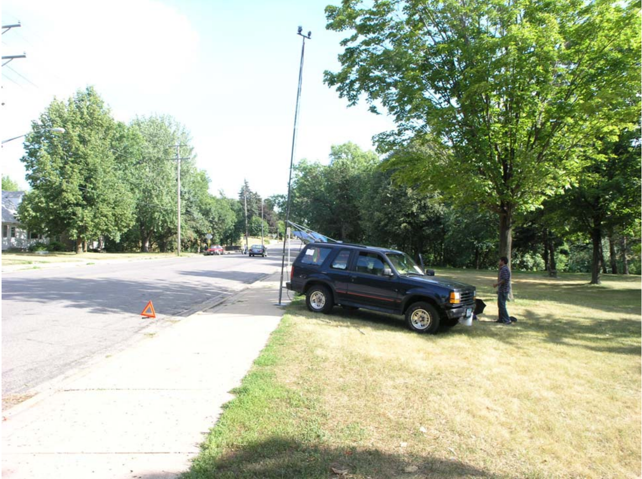
Figure 2. Photograph of camera boom erected at an observation site.
