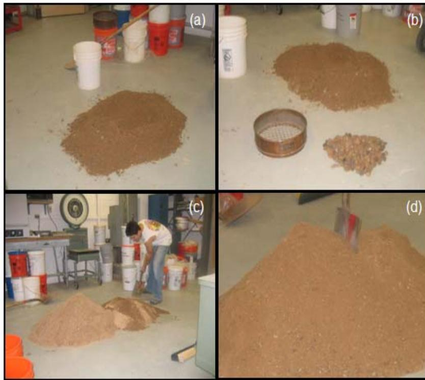
**Fig. C.2. Different stages of RSG production: Class 5 base (a), material retained (b), mixing with fines (c), and final RSG blend (d).**
