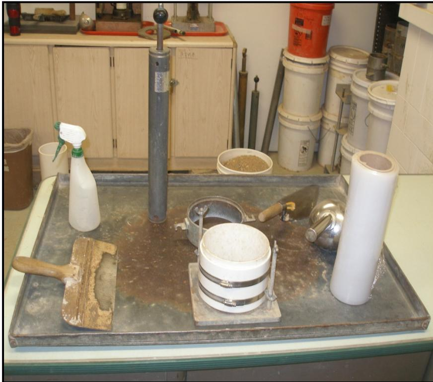
**Fig. D.1. Compaction testing equipment.**
