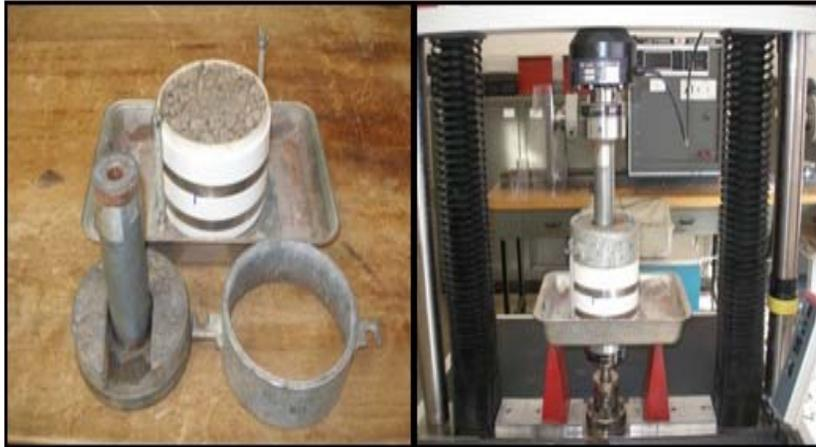
**Fig. D.2. CBR testing equipment.**
