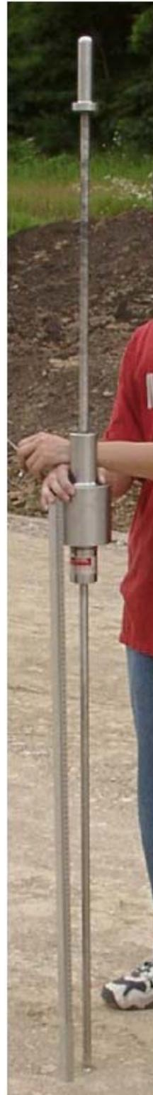
**Fig. 3.5. Dynamic Cone Penetrometer (DCP)**
