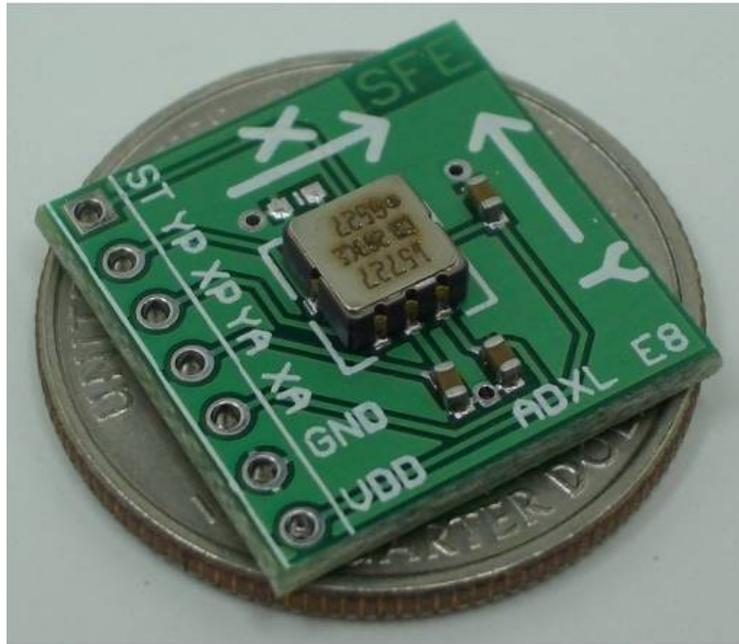
**Fig. A.2. Analog Devices ADXL 203CE accelerometer and corresponding printed circuit board (PCB, Sparkfun Electronics), (adopted from Schuettpelz, 2008).**
