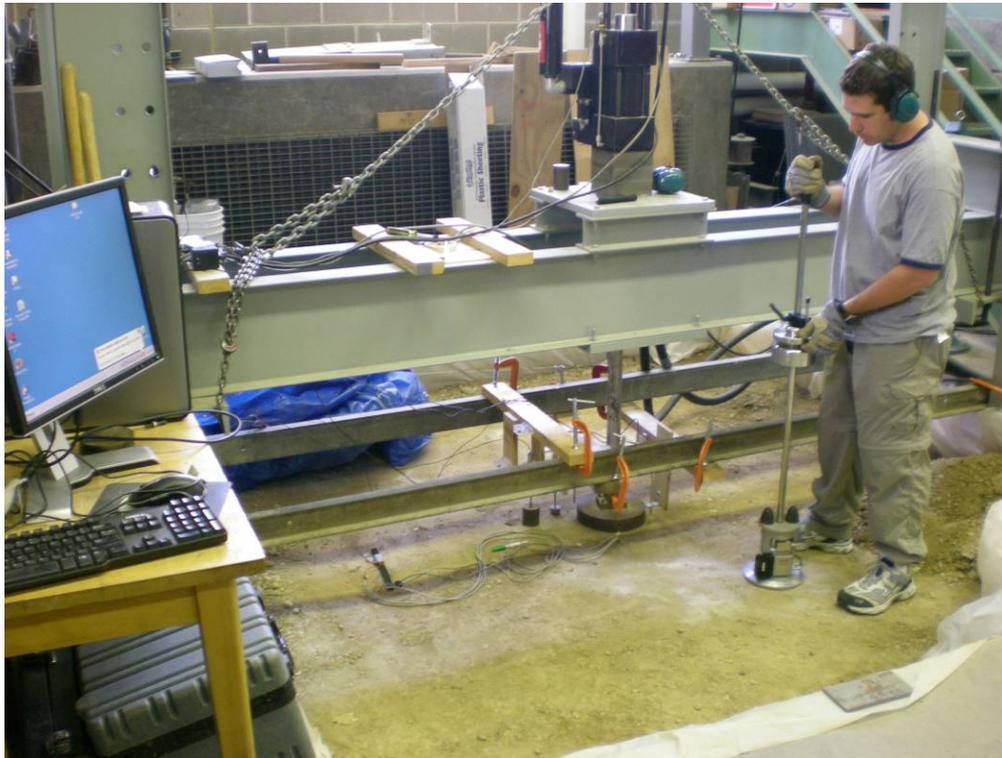
**Fig. 3.4. Measurement of Elastic Modulus with a Keros 100 LWD.**
