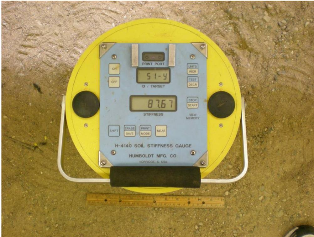
**Fig. 3.3. SSG Displaying an Elastic Modulus Measurement of Class 5 Gravel.**
