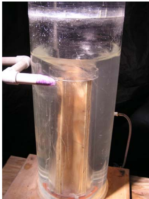
Figure 4-5: A wooden cross baffle inserted inside the inner cylinder
