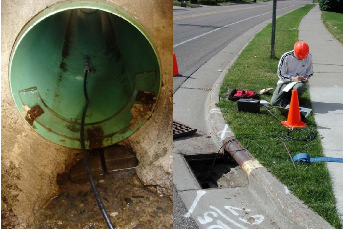
Figure A-4: Flow rate measurement using a weir, pressure transducer and data acquisition computer
