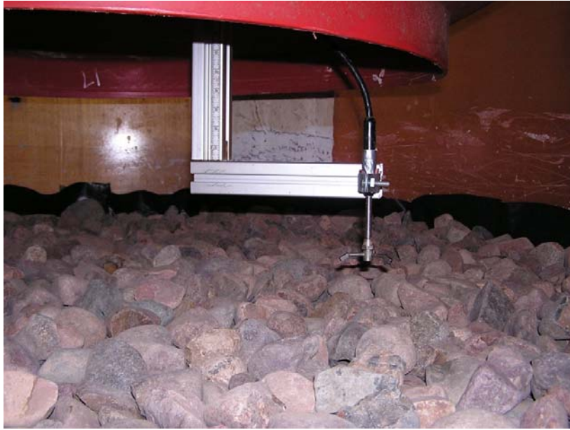
Figure 5-6: ADV positioned above the river rock bed
