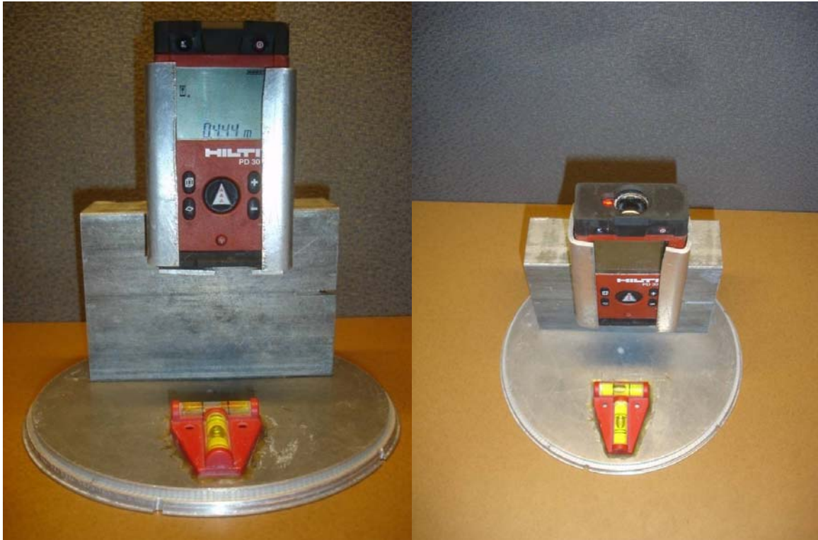
Figure C-2: Laser range finder with bracket
