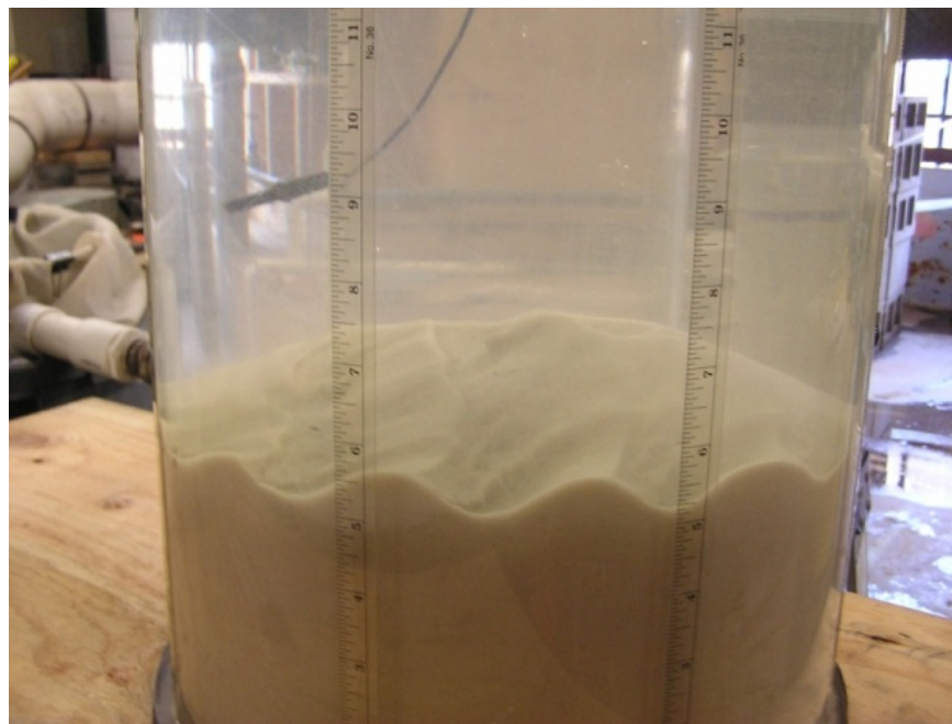
Figure 4-2: Bedforms in swirl flow device scale model
