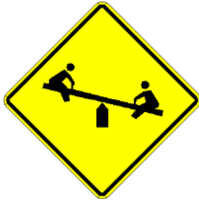
Figure 2.1. Occasional Hazard (Playground) Warning Sign (1)
