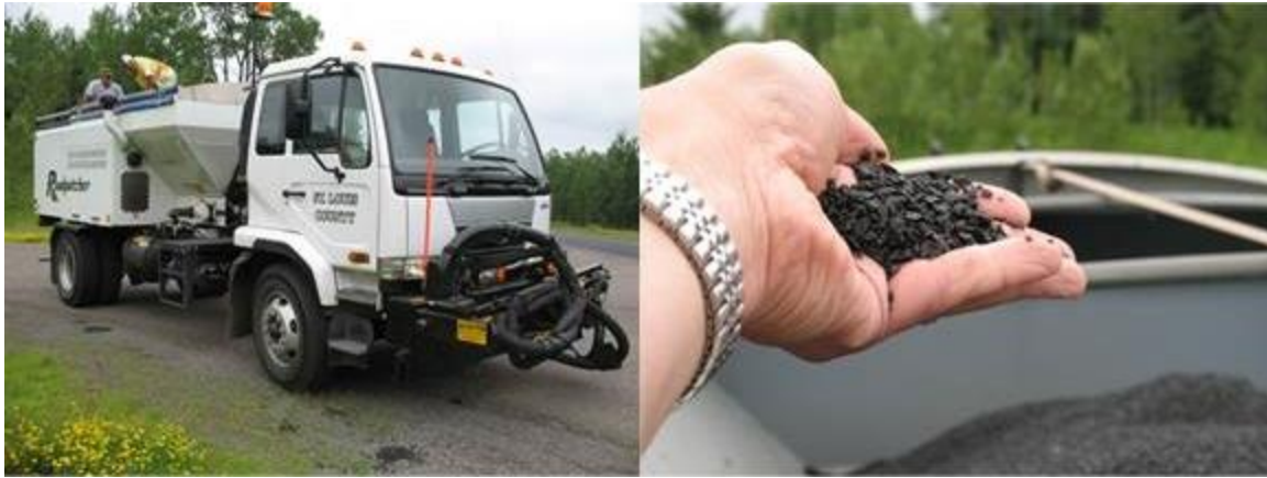
Figure 2.2. Spray patch vehicle (left) and coated aggregate used for patching (right).
