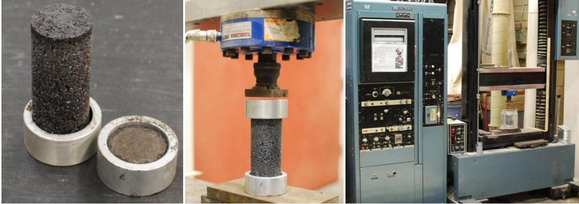
Figure 2.12. Setup of Universal Testing Instrument for performing unconfined compression test.
