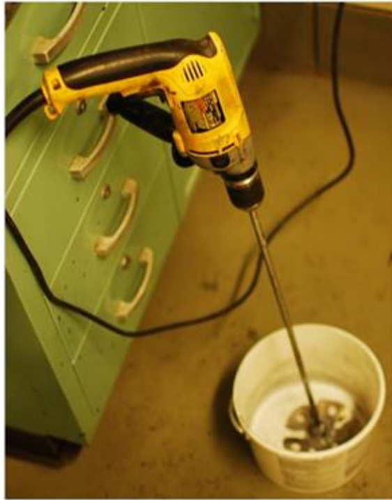
Figure 2.10. Drill, paddle, and mixing bucket used for Rapid Patch lab test work.
