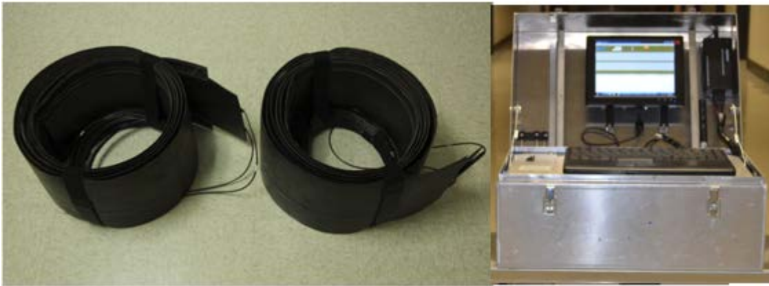
Figure 1: A pair of weigh-pads and PWIM controller
