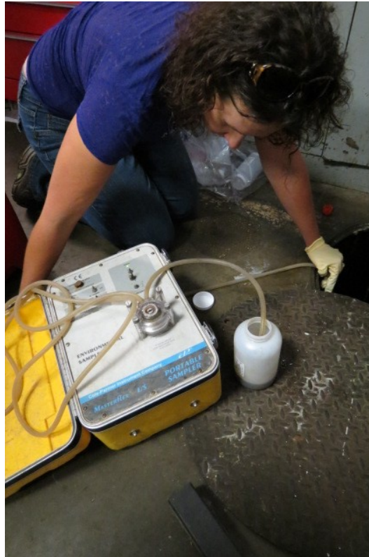
Figure 3.3 Sampling the flammable waste trap with the Masterflex E/S Sampler at the Arden Hills Truck Station during a truck washing event.
