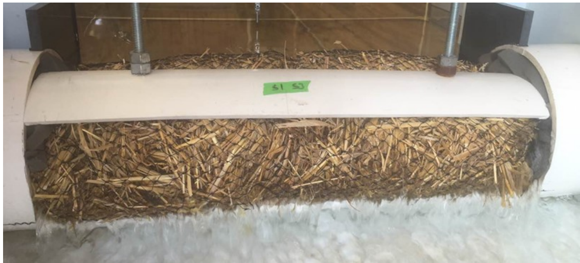
Figure 1 Sediment Control Log with Straw (S1, Western Excelsior Straw)
