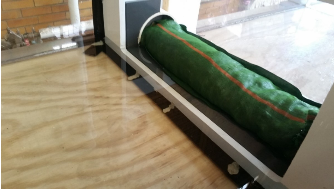
Figure 4 Sediment Control Log with River Pebble Rocks.
