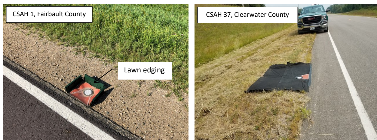
Figure 3.4 Photographs showing the installation of lawn edging (CSAH 1, Fairbault County; photo courtesy: William Goo), and geotextile fabric (CSAH 37, Clearwater County; photo courtesy: Dan Sauve) installed around the runoff sampler during 2018 monitoring. All sites were switched to geotextile fabric cover in 2019.
