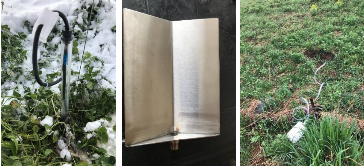
Figure 2.7 The suction lysimeter (left) used in 2019 and the 1-ft pan lysimeter (middle and right) used in 2020 at the Eagle's Nest slope.
