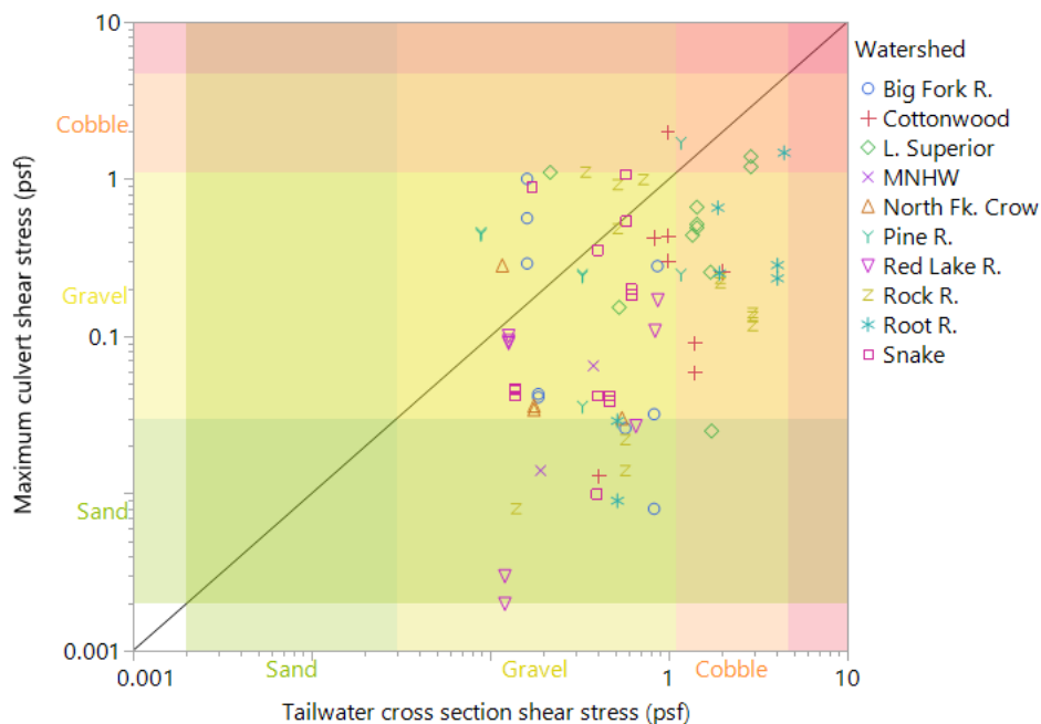
Figure 28. Modeled maximum culvert shear stress compared to the modeled tailwater shear stress for Q1.5. The diagonal line is the 1:1 relationship. Colors represent ranges of critical shear stress for sediment size classes (Fischenich 2001).
