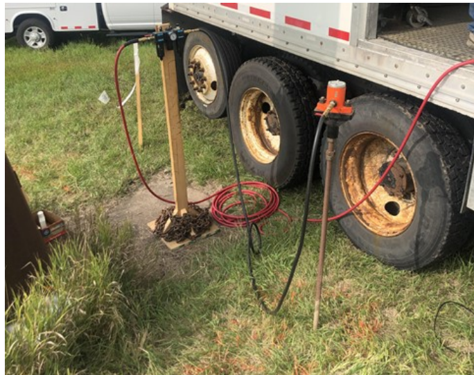
Figure 2.2 Pneumatic vibratory shaker device configuration.
