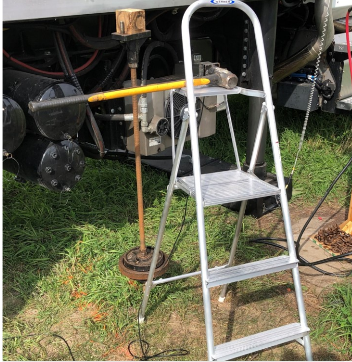
Figure 2.6 Hammer impact method configuration.
