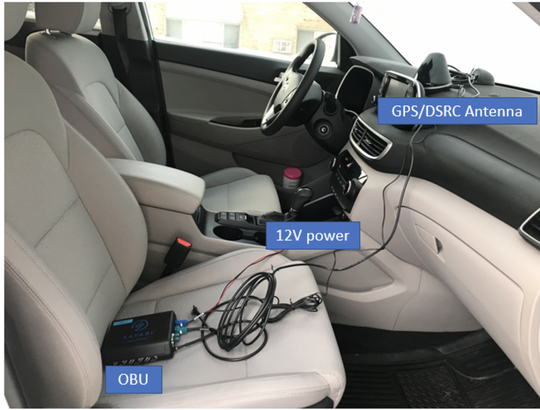
Figure 9.1: OBU installation inside a vehicle
