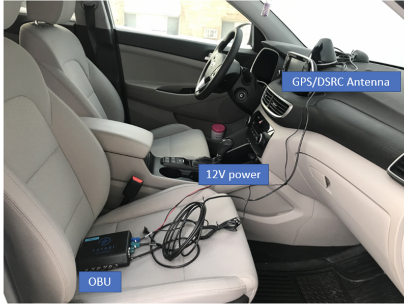
Figure 2.2: OBU installation diagram
