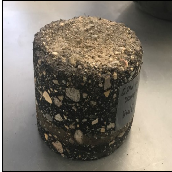
Figure 4-8 Bottom surface of field cores
