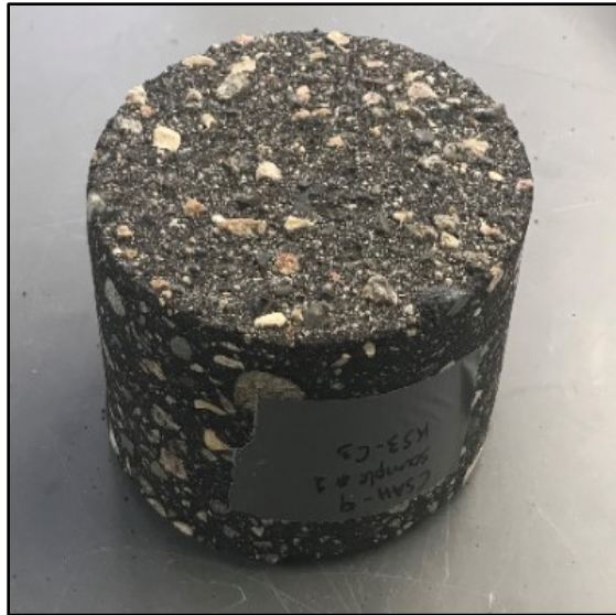
Figure 4-7 Top surface of field cores
