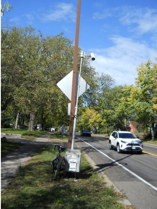
Figure 3.1 MTO's Pole-Anchored Camera at Our Louisiana/Franklin Site.
