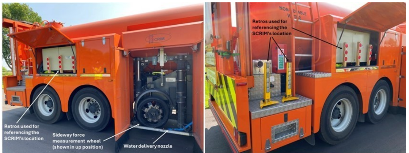
Figure 5.6 SCRIM vehicle components showing two types of retros.
