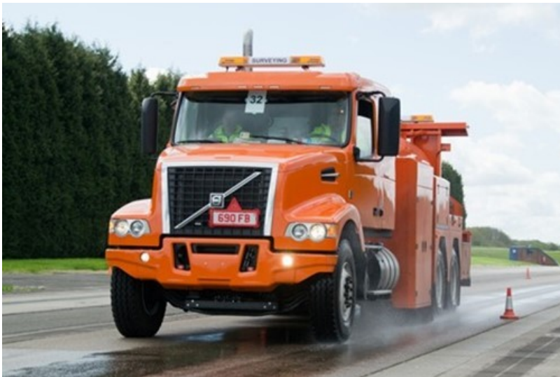
Figure 5.5 SCRIM vehicle (image source: WDM)
