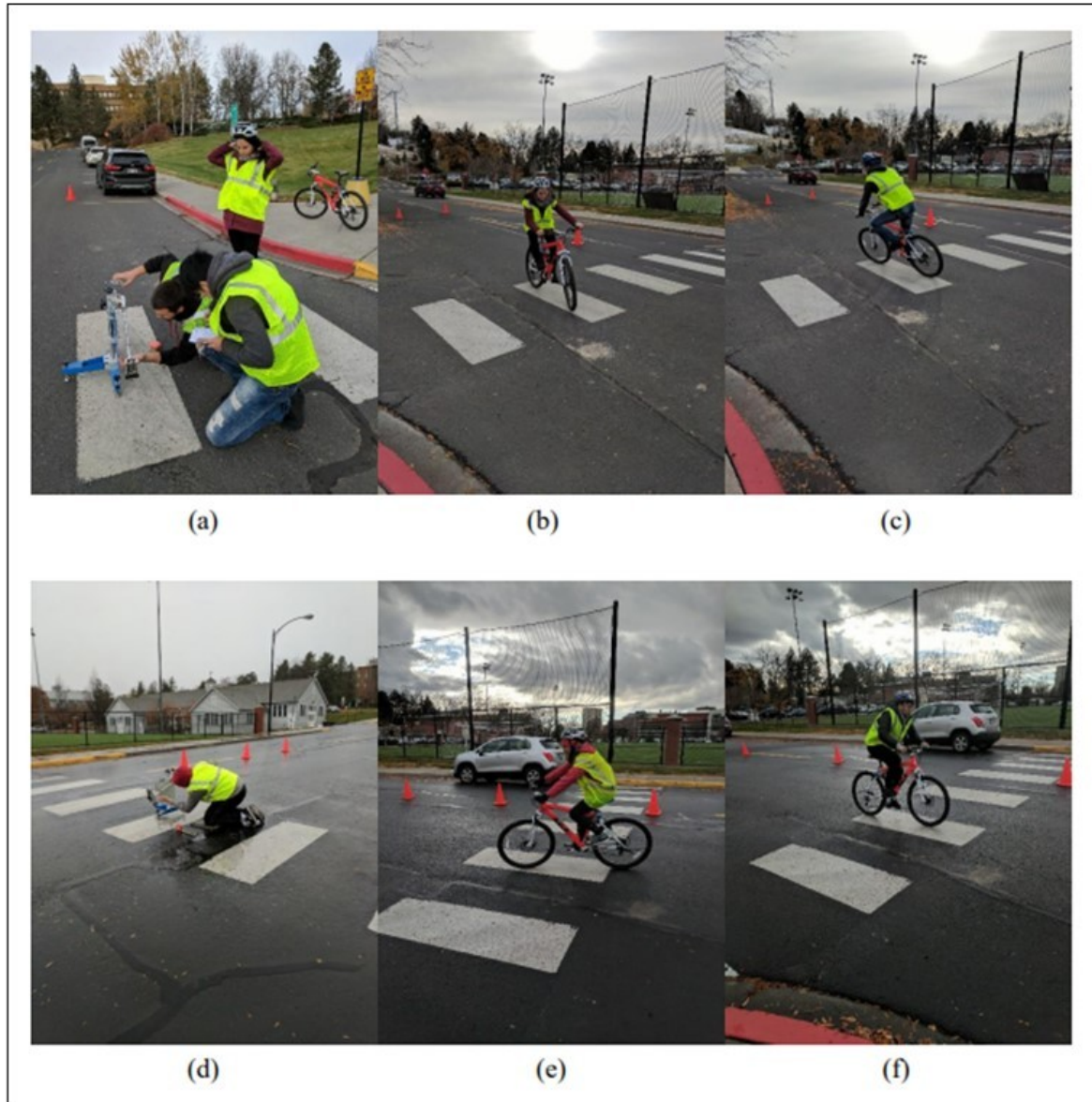
Figure 2.5 Dry testing using the mountain bike at Test Site 1 by a) the BPT, b) rider one, and c) rider two. Wet testing at Test Site 2 by d) the BPT, e) rider one, and f) rider two (Nassiri, 2018)
