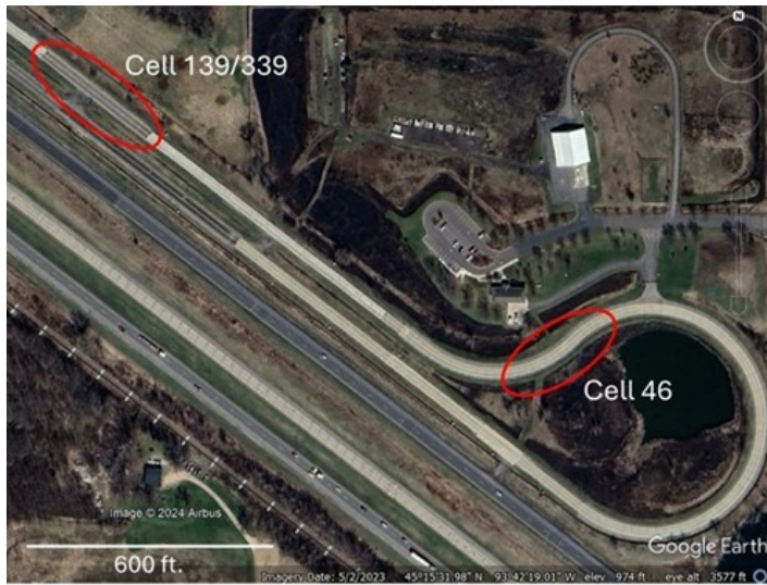
Figure 5.2 Google Earth image of MnROAD Low Volume Road cells for pavement markings testing (Cell 46 concrete; Cell 139/339 asphalt)
