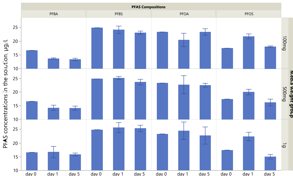
Figure 19. The concentrations of four PFAS species at the beginning (day 0), the first day (day 1) and the fifth days (day 5) during the adsorption test.: 100 mg (top), 500 mg (middle) and 1 g (bottom) of TDA were added to 40 ml of water containing the PFAS species with triple replicates for each.
