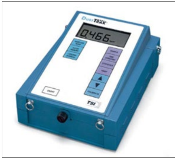
Figure 6.3. DustTrak Model 8520 (image source: TSI)
