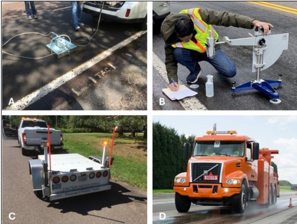
Figure 7.26. Data collection methods/equipment and respective operating parameters: A) Dynamic Friction Tester; B) British Pendulum; C) MnDOT's Locked-Wheel Pavement Friction Tester; and D) Sideway-force Coefficient Routine Investigation Machine (SCRIM)
