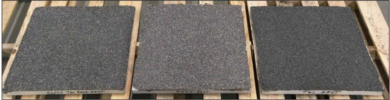
Figure D.1. Test slabs with HFST application
