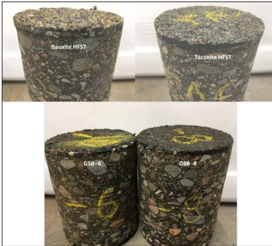
Figure 7.16. Cores collected from the four pavement treatment test sections
