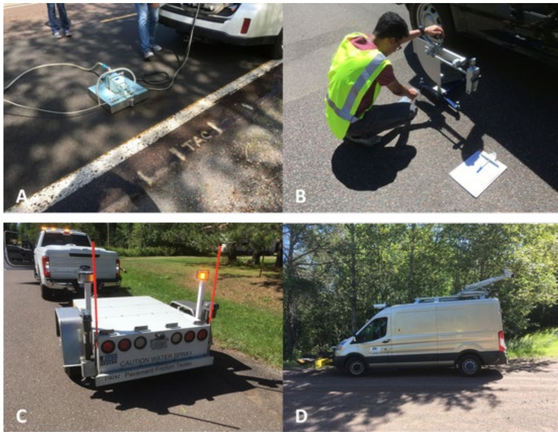
Figure 7.1. Data collection methods/equipment: A) Dynamic Friction Tester; B) British Pendulum; C) MnDOT's Locked-Wheel Pavement Friction Tester; and D) MnDOT's Road Doctor
