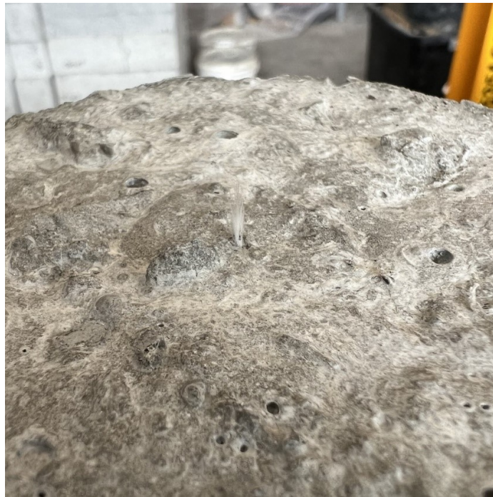
Figure 6.17: Fiber 2 (failure at concrete interface)
