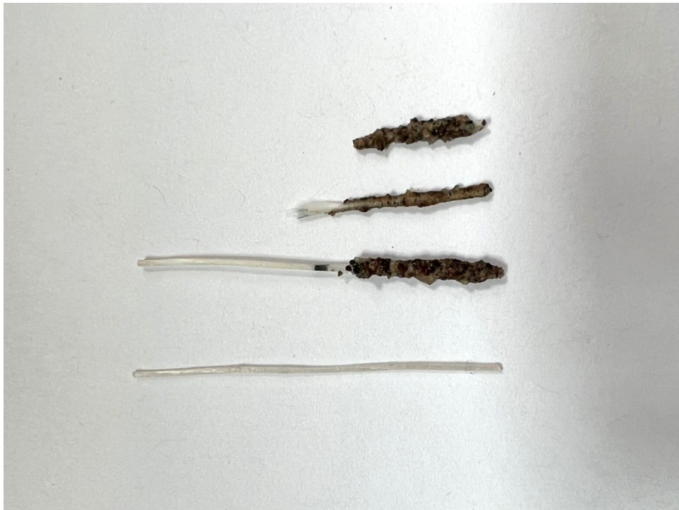
Figure 6.15: Fiber 2 (failed fibers vs new fiber)
