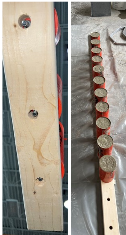
Figure 6.2: Casting platform with cylinders installed.
