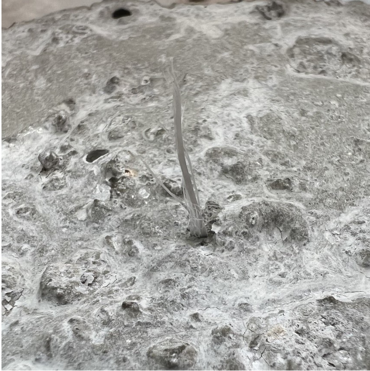
Figure 6.23: Fiber 4 (failure at the concrete interface).
