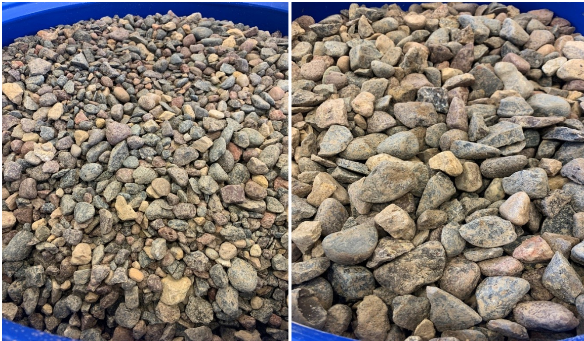
Figure A-16 Class C aggregate (3/4" on left, 1.5" on right)
