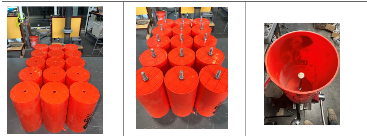
Figure 6.1: Plastic mold arranged for the single fiber pullout test sample preparation.
