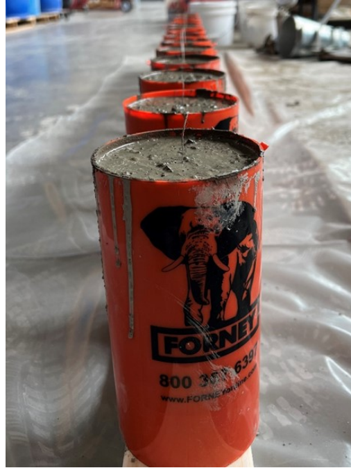
Figure 6.3: Embedded fibers in fresh concrete cylinders.
