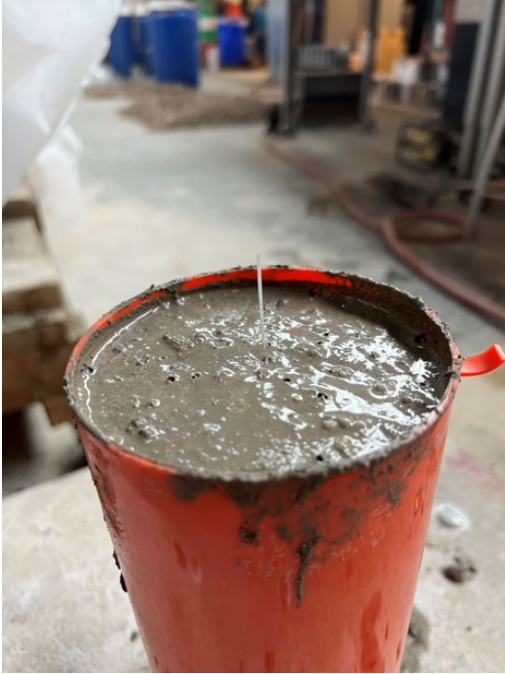
Figure 6.3: Embedded fibers in fresh concrete cylinders.
