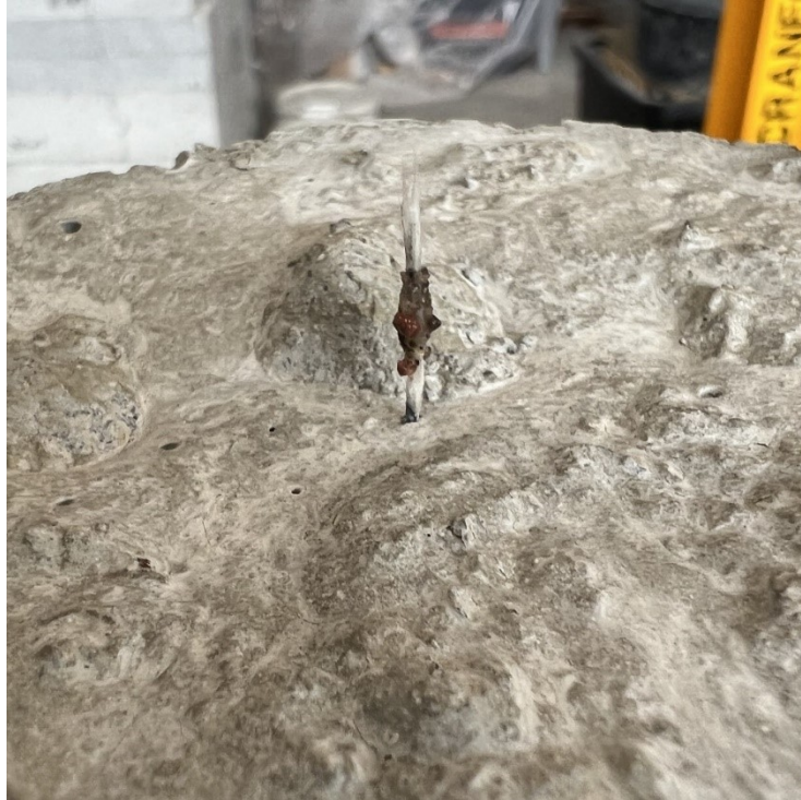
Figure 6.16: Fiber 2 (failure at grip interface)
