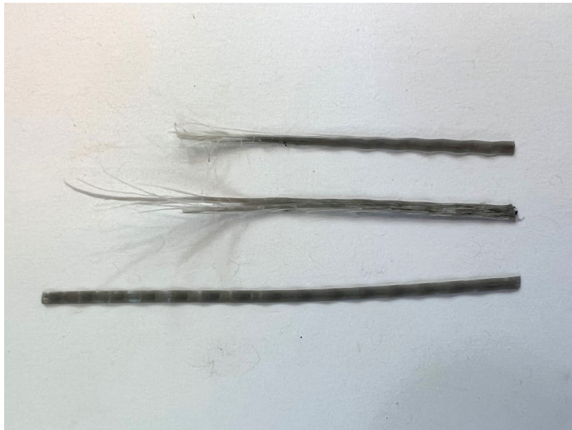
Figure 6.22: Fiber 4 (failed fibers compared to original fiber).
