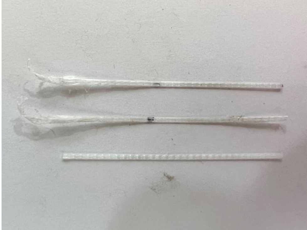
Figure 6.13: Fiber 1 (failed fibers vs new fiber).
