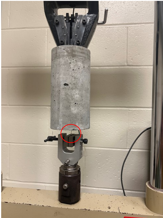
Figure 6.4: Single fiber pullout test in progress.
