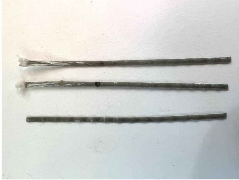
Figure 6.21: Fiber 4 (failed fibers vs new fiber).
